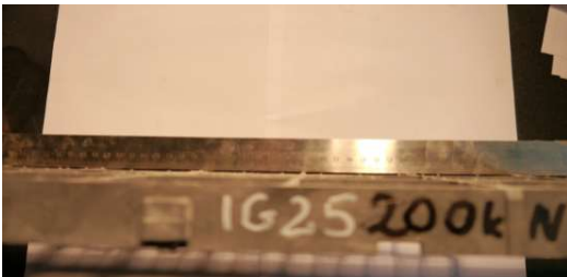
Photo.5. IG 25 after the test at 200 kN
